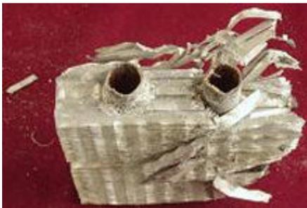
Macro photo of conventional copper tube-aluminum fin heat exchanger before and after one year in a coastal environment!
